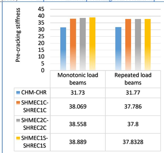
Fig. 18. Effect variables on pre-cracking stiffness value.
