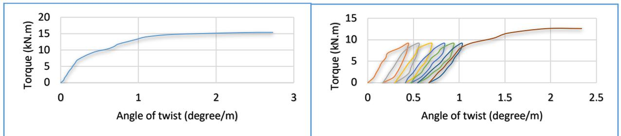
(a) Beams tested under Monotonic loads.
