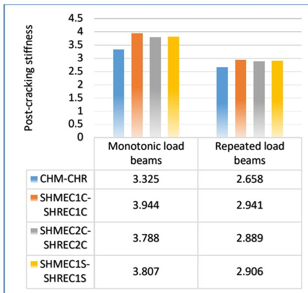
Fig. 19. Effect variables on post-cracking stiffness value.
