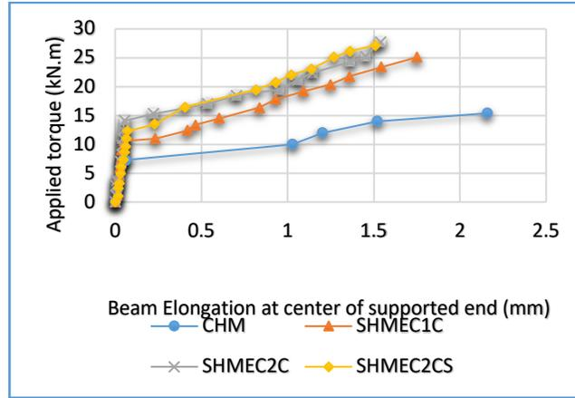
Fig. 13. Beam longitudinal elongation tested under monotonic loads.
