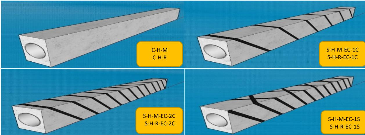
Fig. 3. strengthening scheme of the tested beams.
