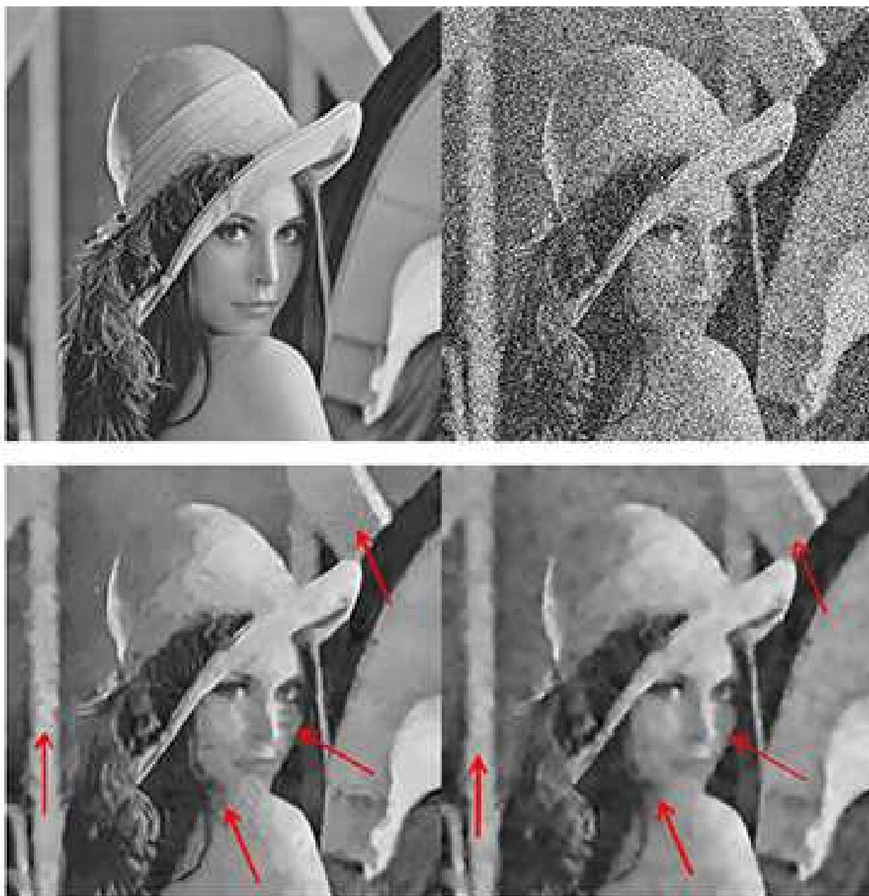
Fig. 9: First row: "Lena" image and that with AWG noise, \sigma = 100 ; Second row: Results by BM3D and LFAD. Arrows show areas where LFAD performs comparatively better than BM3D.
