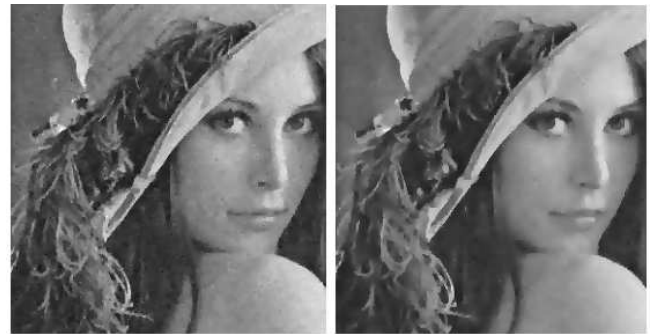
Fig. 2: PM denoised "Lena" image for two different iteration numbers (left = 22 iterations, PSNR = 29.37 dB; right = 30 iterations, PSNR = 28.52 dB) for AWG noise level, \sigma = 20 .
