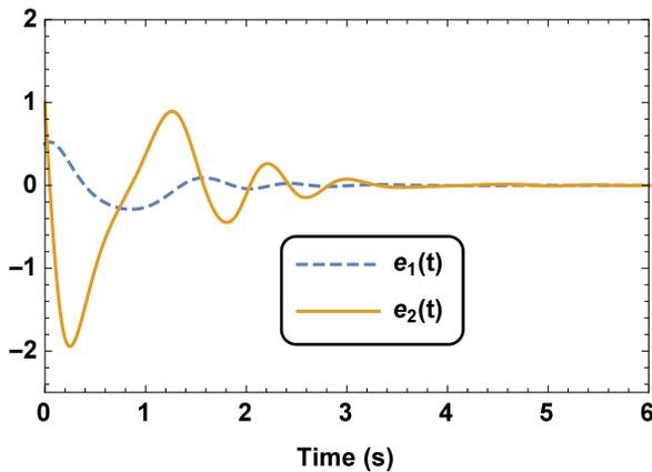
Fig. 4: Time series of the trajectories  $e_1(t)$  and  $e_2(t)$  of the error system tend to zero
