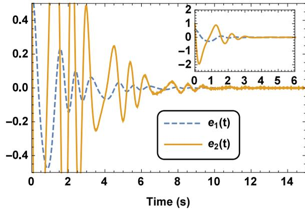
Fig. 8: Time series of the synchronized error states for two identical chaotic gyros under the effect of unknown external disturbance
