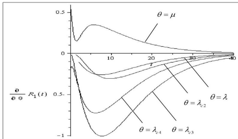
**Fig. 8:** Sensitivity of the reliability of configuration I with respect to system parameters.
