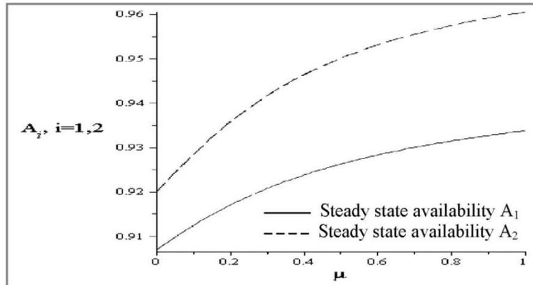
**Fig. 7:** Steady state availability  $A_i$  versus repair rate  $\mu$ ,  $i=1,2$
