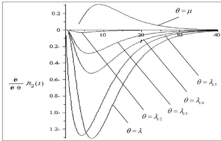
**Fig. 9:** Sensitivity of the reliability of configuration II with respect to system parameters
