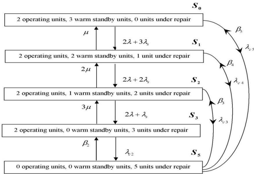
**Fig. 3:** State transition diagram of 2-out-of-5:G warm standby parallel repairable system
