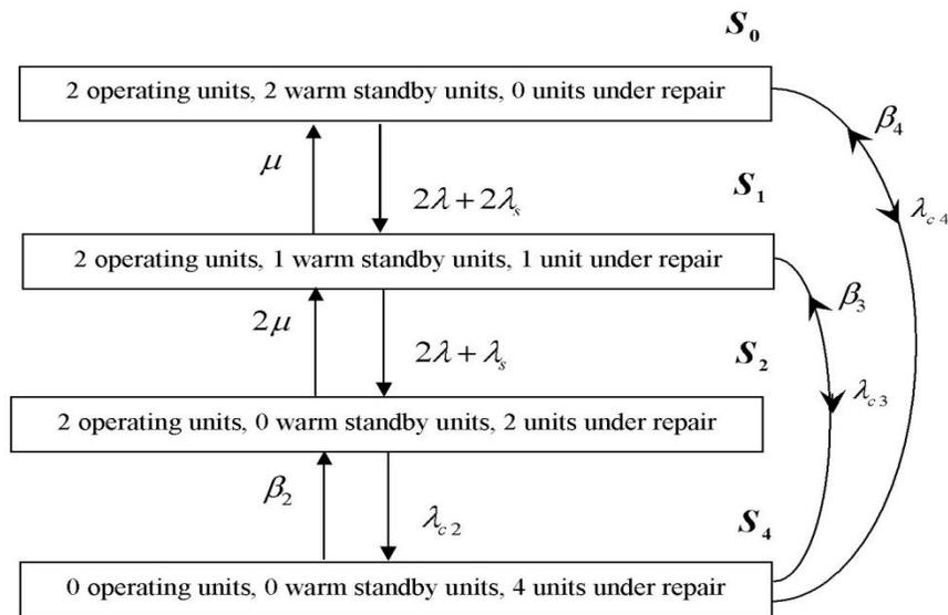
**Fig 2:** State transition diagram of 2-out-of-4:G warm standby parallel repairable system
