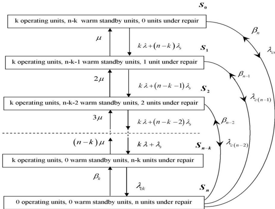
**Fig. 1:** State transition diagram of the k-out-of-n:G warm standby parallel repairable system
