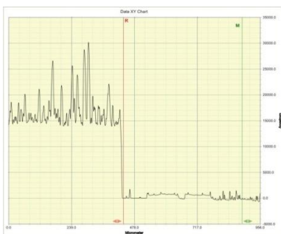
Figure 2c: Surface profile of the as-deposited CuSbS 2 thin film obtained at 36hr dip time.
