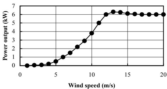
Fig. 5: Power output of WT as a function of wind speed [30].
