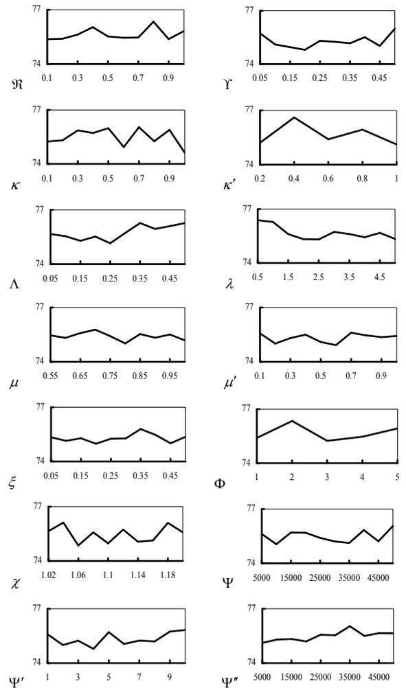
**Fig. 4:** Sensitivity analysis of EICA parameters including constants and coefficients: vertical axis represents the ACS ( $\times 10^3$ ) (\$) and horizontal axis provides the range of values examined.
