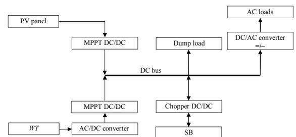
Fig. 1: Autonomous HGPS schematic diagram.
