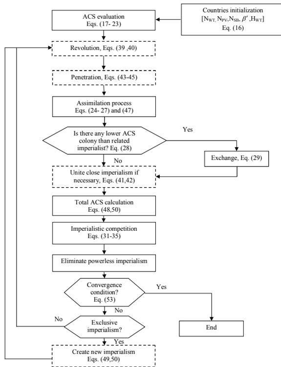
**Fig. 2:** Flowchart for ICA and EICA. The EICA enhancements introduced in this study are shown with dashed line blocks.
