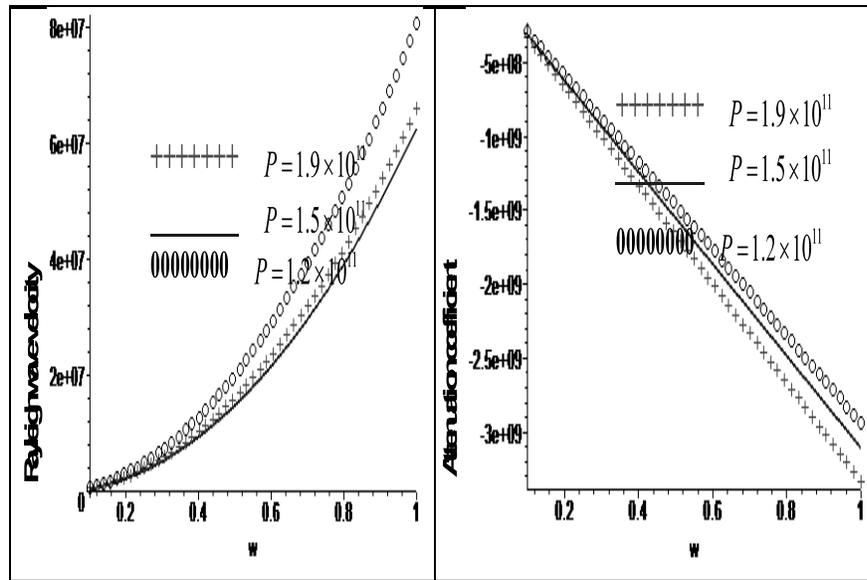
**Fig. 10:** Variation of Rayleigh wave velocity (Re) and attenuation coefficient (Im) for different values of initial stress with respect wave number  $\omega$ .
