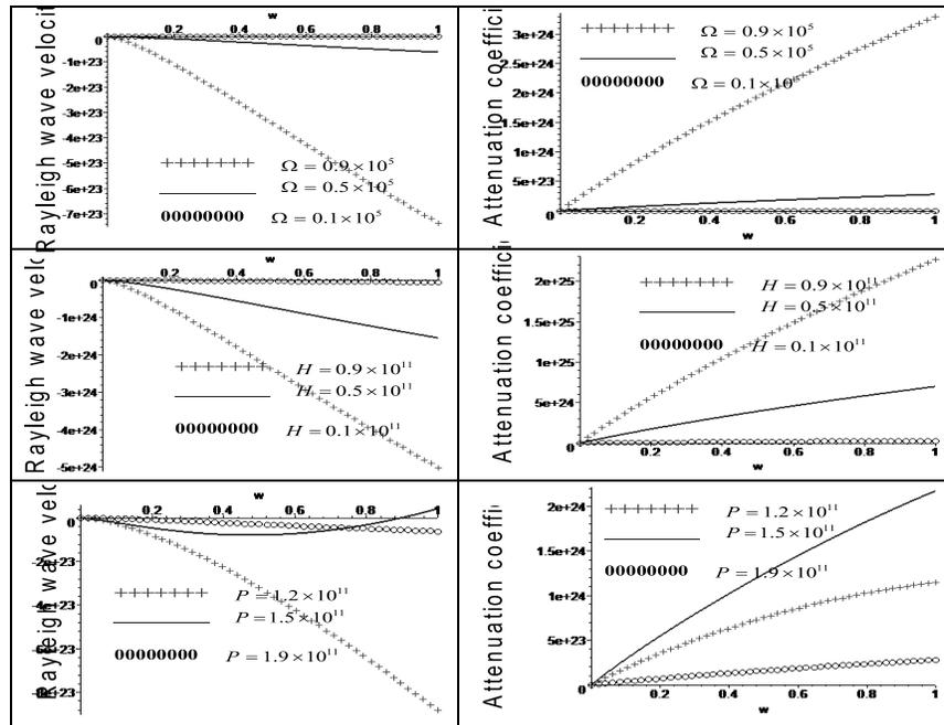
**Fig. 2:** Variation of Rayleigh wave velocity (Re) and attenuation coefficient (Im) for different values of magnetic field, rotation and initial stress with respect wave number  $\omega$ .
