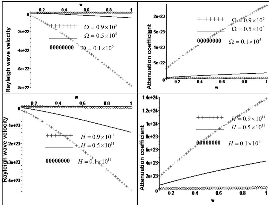
**Fig. 8:** Variation of Rayleigh wave velocity (Re) and attenuation coefficient (Im) for different values of rotation and magnetic field with respect wave number  $\omega$ .
