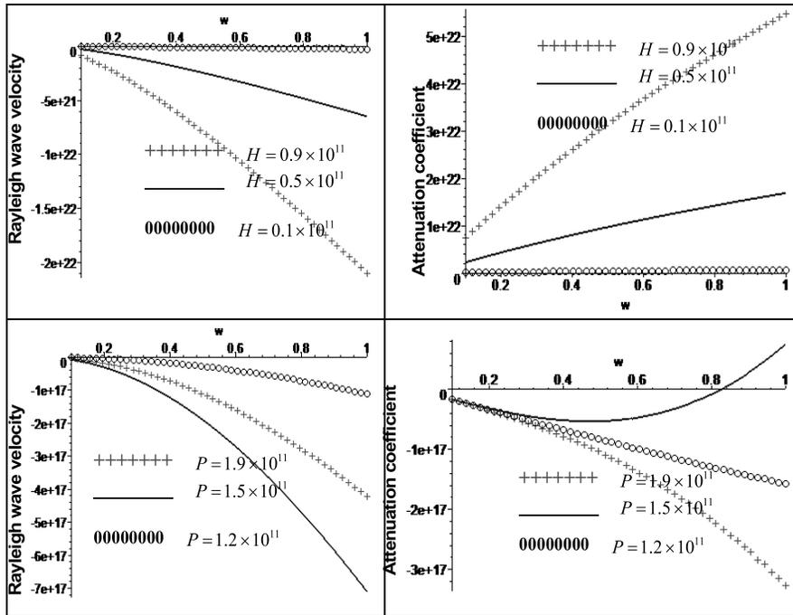
**Fig. 4:** Variation of Rayleigh wave velocity (Re) and attenuation coefficient (Im) for different values of magnetic field and initial stress with respect wave number  $\omega$ .
