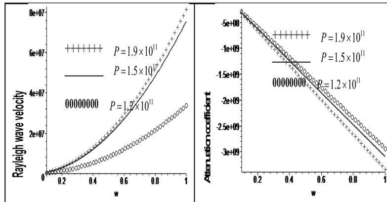
**Fig. 9:** Variation of Rayleigh wave velocity (Re) and attenuation coefficient (Im) for different values of initial stress with respect wave number  $\omega$ .
