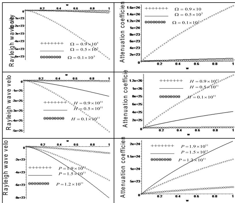
**Fig. 1:** Variation of Rayleigh wave velocity (Re) and attenuation coefficient (Im) for different values of magnetic field, rotation and initial stress with respect wave number  $\omega$ .
