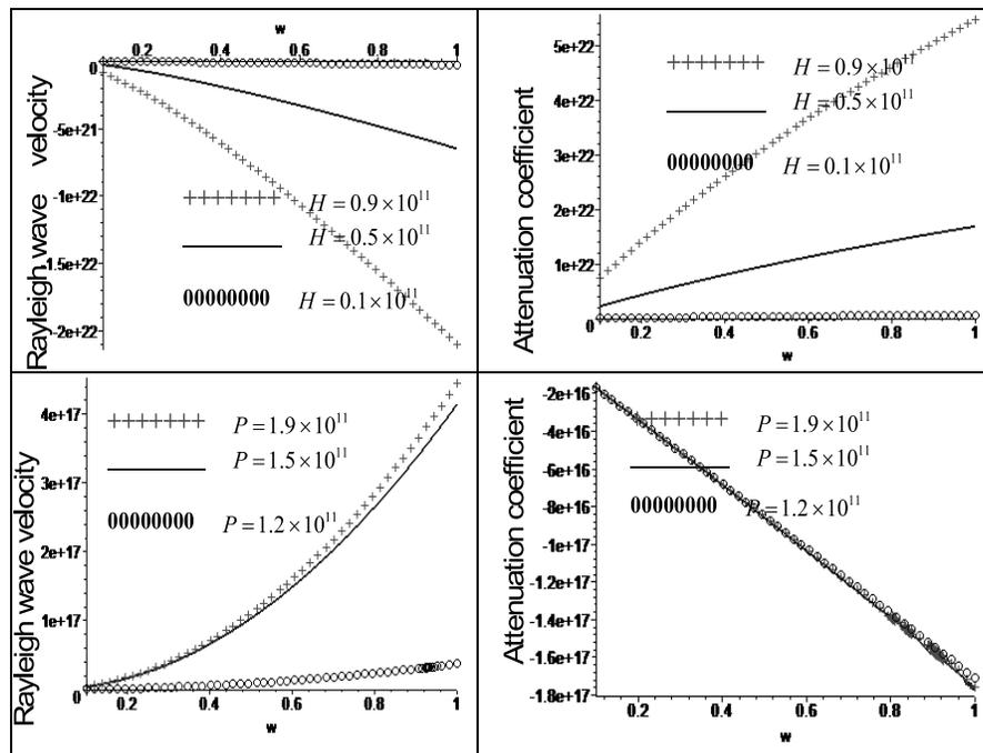
**Fig. 3:** Variation of Rayleigh wave velocity (Re) and attenuation coefficient (Im) for different values of magnetic field and initial stress with respect wave number  $\omega$ .
