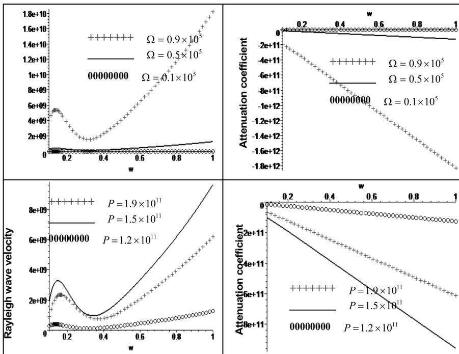
**Fig. 5:** Variation of Rayleigh wave velocity (Re) and attenuation coefficient (Im) for different values of rotation and initial stress with respect wave number  $\omega$ .
