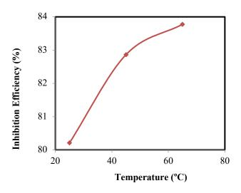
Figure 4. Inhibition efficiency of the extract in HCl at different temp. degrees
