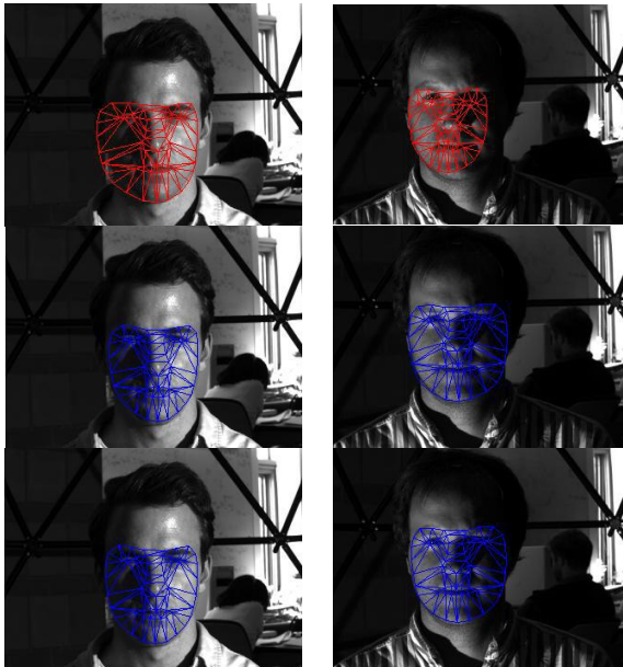
Figure 5: AAM fitting for the original AAM (Top), the DoG kernel (Middle) and Canny edge (Bottom) using Yale face database to evaluate performance against diverse illuminations.
