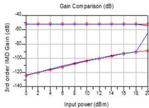
Fig. 12: 3 rd order IMD Gain reconstruction of actual and modeled PA
