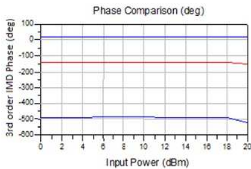
Fig. 13: 3 rd order IMD Phase reconstruction of actual and modeled PA
