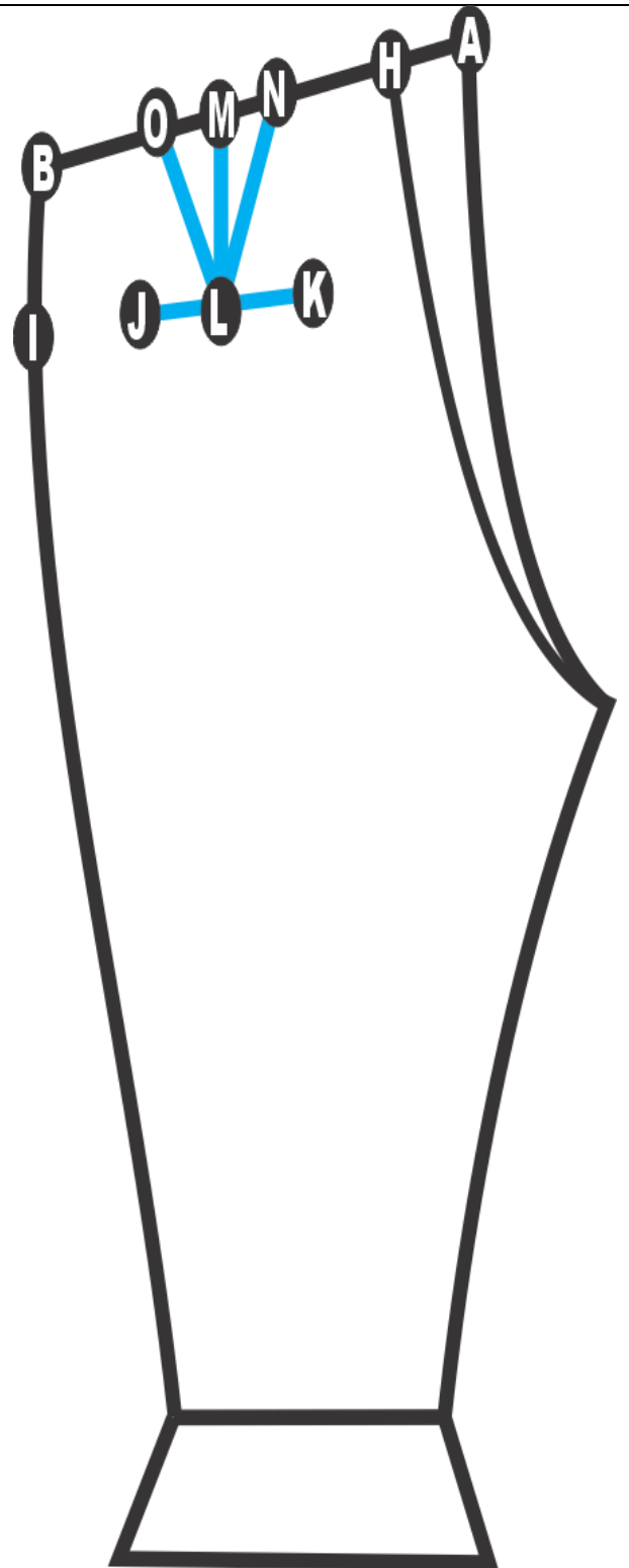
Figure 118: Method 2 of drafting a dart and hip pocket
