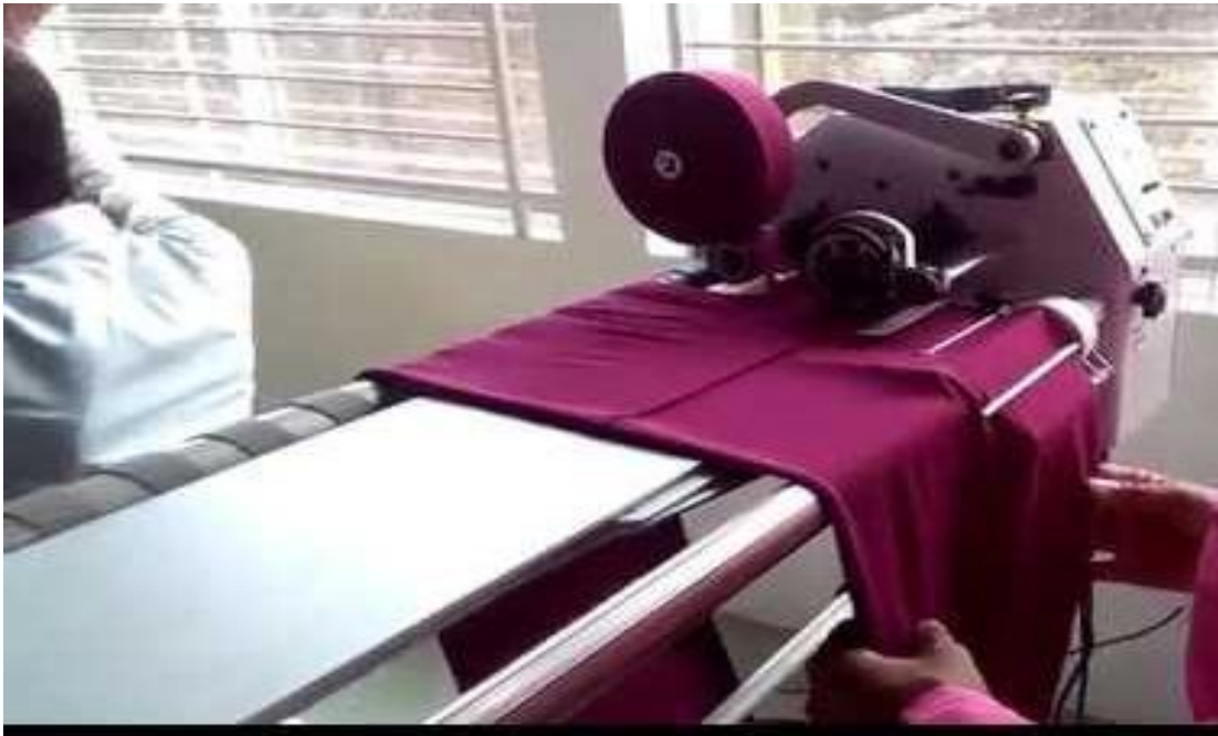
Figure 25: Rib cutting machine
