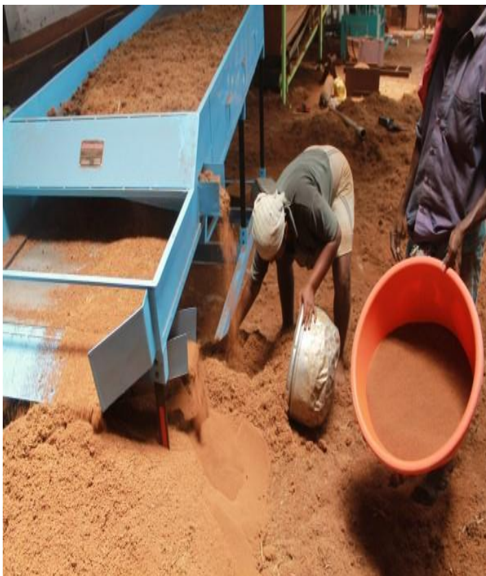
Figure 86: Sieving, or screening coir
