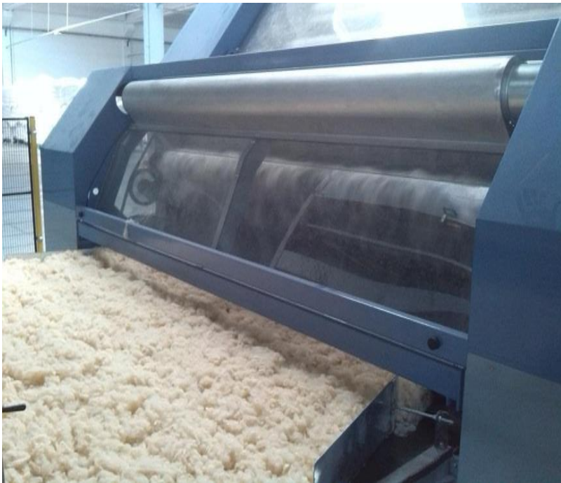
Figure 115: Carding of asbestos
