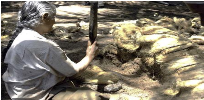
Figure 82: Manual decortivating of coir
