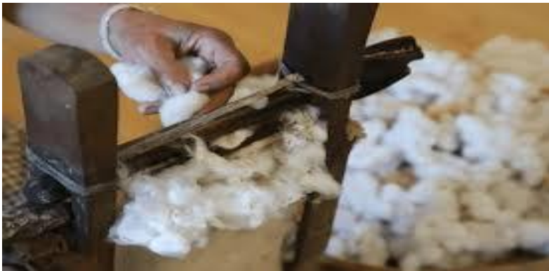
Figure 4: Manual ginning of cotton
