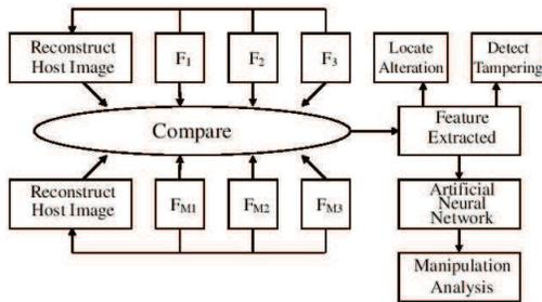
**Fig. 5:** Fragile watermark extraction and analysis.
