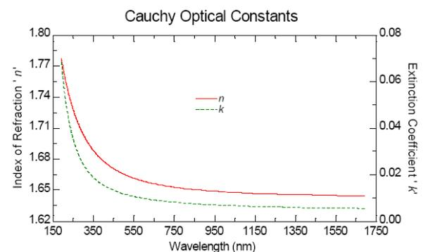
**Fig. 3:** Refractive index ( $n$ ) and extinction coefficient ( $k$ ) as a function of the wavelength for the bulk-like aluminum oxide layer of sample A432-b.
