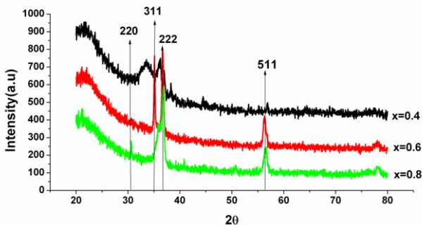
**Figure 4.** XRD pattern of  $Mn_xZn_{1-x}Fe_2O_4$  thin films.
