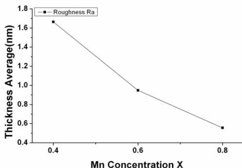
**Figure 8.** Roughness average of  $Mn_xZn_{1-x}Fe_2O_4$  thin films.
