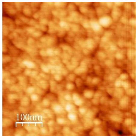
**Figure 7.** AFM images of  $Mn_xZn_{1-x}Fe_2O_4$  thin film ( $x=0.8$ ).
