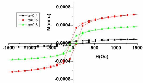
**Figure 9.** M-H loops of  $Mn_xZn_{1-x}Fe_2O_4$  thin films
