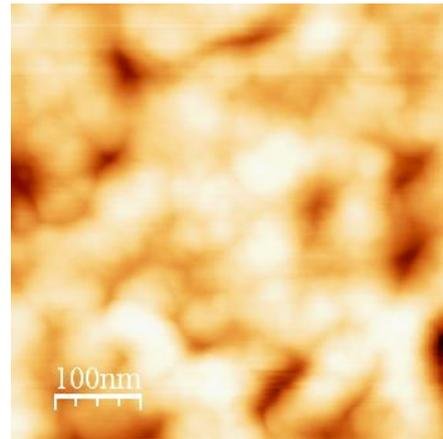
**Figure 5.** AFM images of  $Mn_xZn_{1-x}Fe_2O_4$  thin film ( $x=0.4$ ).
