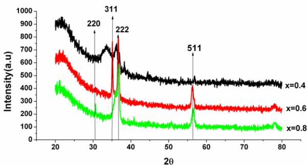
**Figure 4.** XRD pattern of  $Mn_xZn_{1-x}Fe_2O_4$  thin films.
