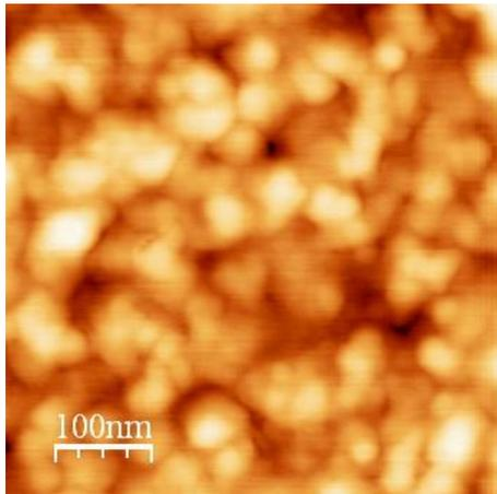
**Figure 6.** AFM images of  $Mn_xZn_{1-x}Fe_2O_4$  thin film ( $x=0.6$ ).
