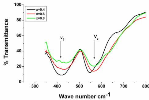
**Figure 2.** FT- IR absorption spectra of  $Mn_xZn_{1-x}Fe_2O_4$
