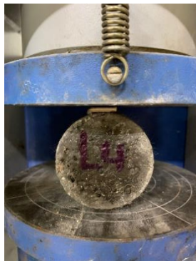
e) Test setup for splitting tensile test
