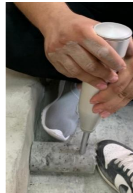
Fig. 25: The pSchmidt hammer test performed in the downward direction on LWFRC cylinders.
