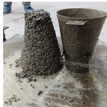
Fig. 10: The slump test for LWFRM mix D12F.
