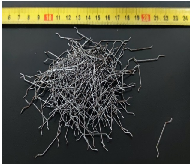
a) End-hook steel fiber
