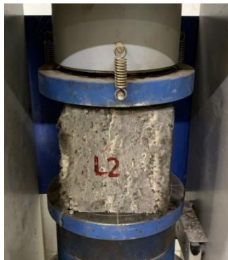
c) Test setup for compression test of the cube
