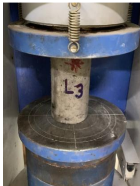
d) Test setup for compression test of the cylinder
