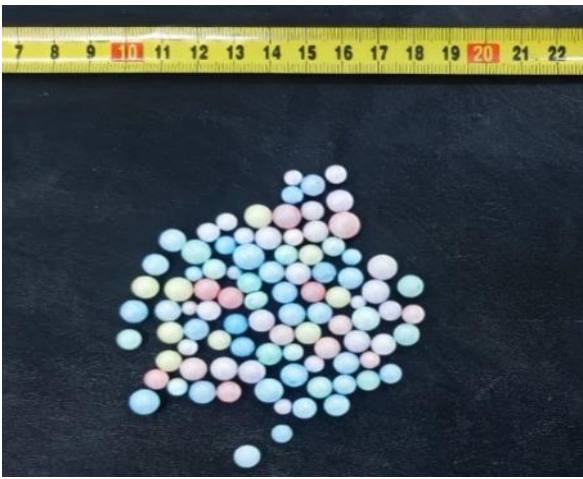
Fig. 4: The size of EPS used in the LWFRM mixes.
