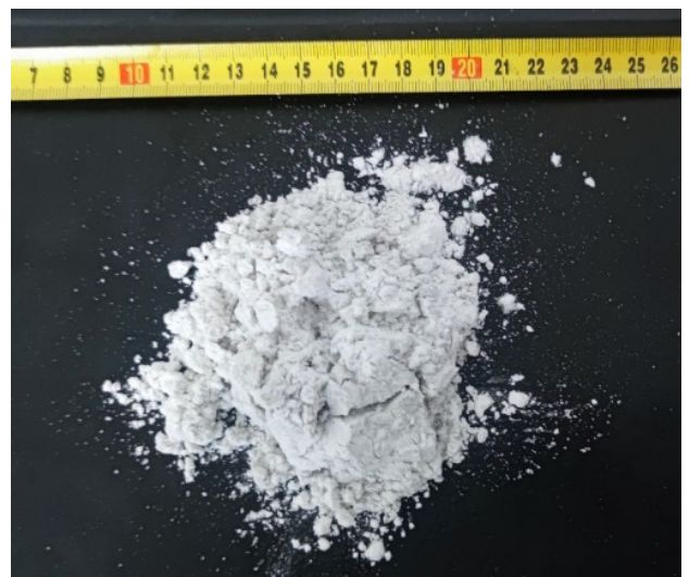
Fig. 3: Fine expanded perlite used in the LWFRM mixes.
