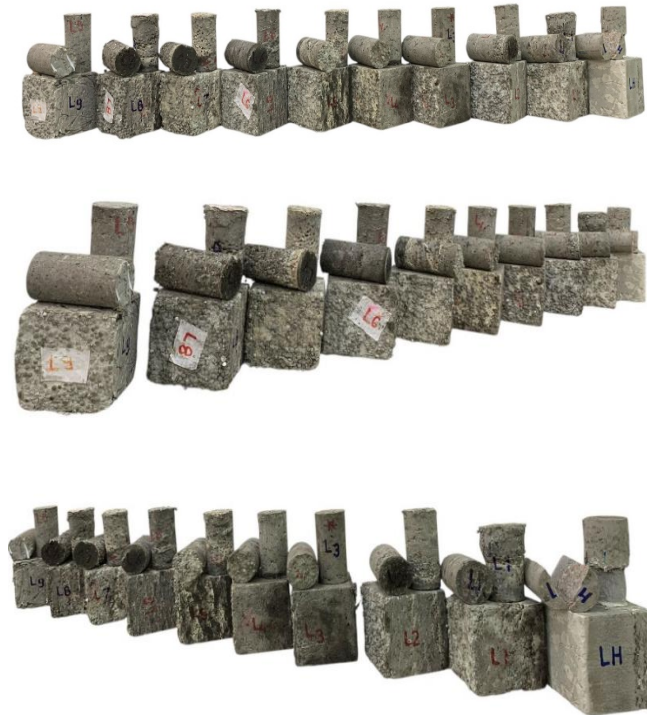
Fig. 14: The fracture formation for all LWFRC mixtures, cubes, cylinders, and splitting in cylinders.
