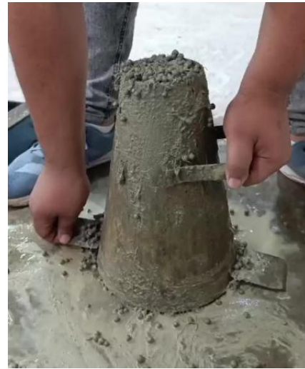
a) Test setup for the slump test
