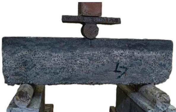
f) Test setup for the flexural tensile strength
