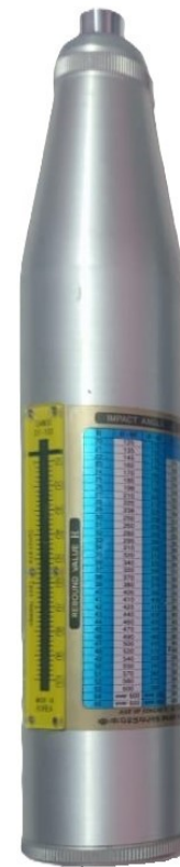
Fig. 9: Schmidt hammer used in this study.
