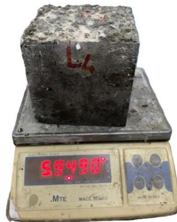
b) Test setup for calculate the density after 28 days
