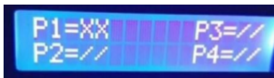
Illustration 8: The current status of the LCD screen indicates that the P1 slot is unavailable at this time
