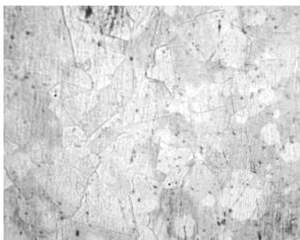
Fig. 2e. Microstructure for sample SS304L.
