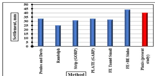
Figure 5. Maximum-settlement relationship for different approaches for the example reported by Poulos<sup>(7)</sup>.
