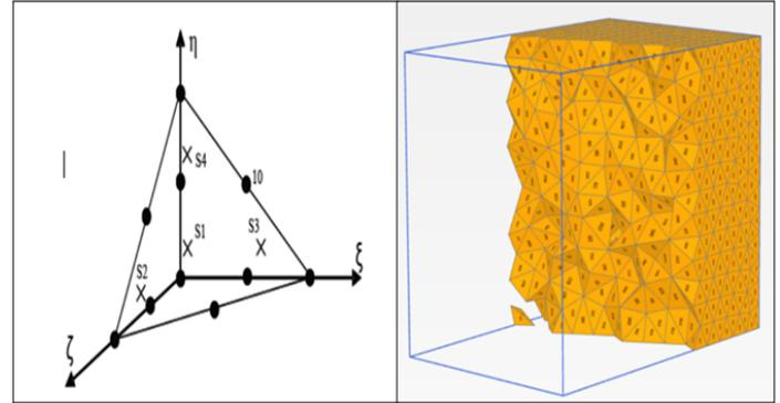
**Figure 7.** 3-D soil element (10-Node Tetrahedron).
