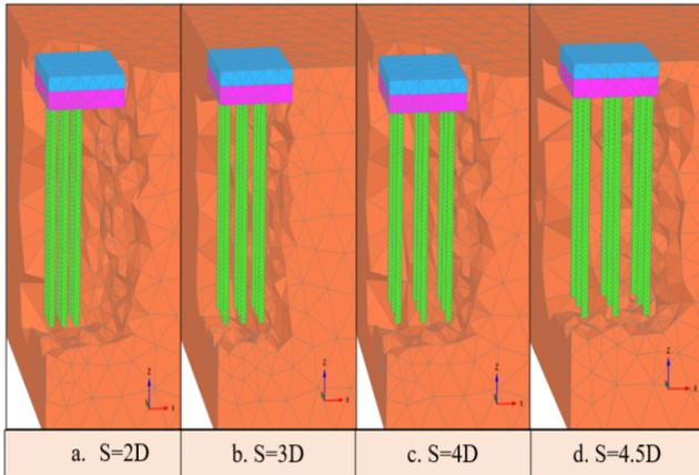
**Fig. 8:** Finite elements mesh of unconnected piled raft foundation with different pile spacing (S).
