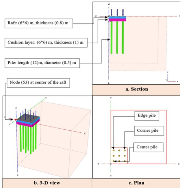
**Figure 6.** One-fourth of the reference unconnected piled raft system.
