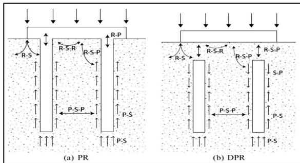
**Fig. 2:** Interactions between soil and structural members (R = raft; P = pile; S = soil), (Tradigo et al., 2016).
