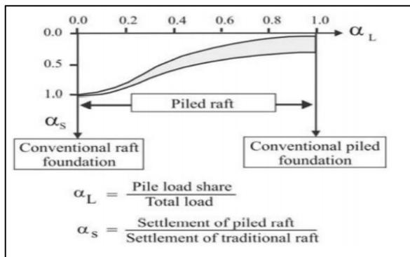
**Fig. 1:**  $\alpha_s$  and  $\alpha_L$  values for piled raft foundation design (El-Mossallamy et al., 2006).
