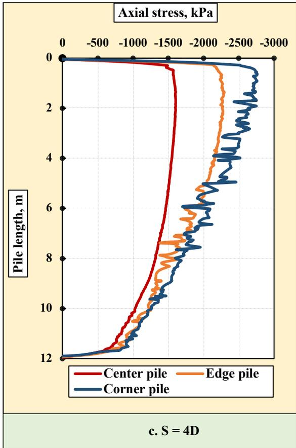
**Fig. 13:** Axial stress along the pile length for different pile spacings (S).
