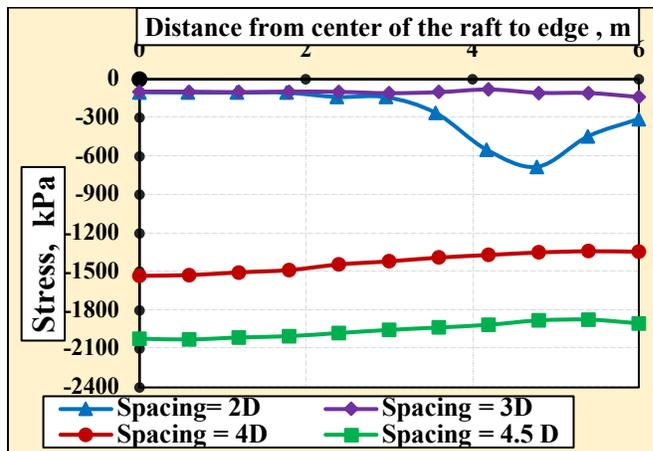
Fig. 12: Effect of the pile spacing on the axial stress along the centerline of the raft.
