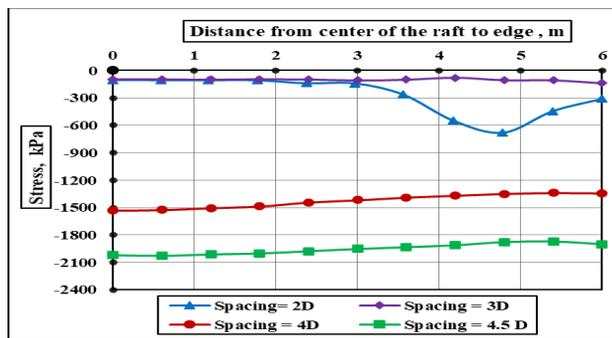
**Fig. 15:** The pile spacing (S) effect on the axial stress parallel to the raft's centerline.
