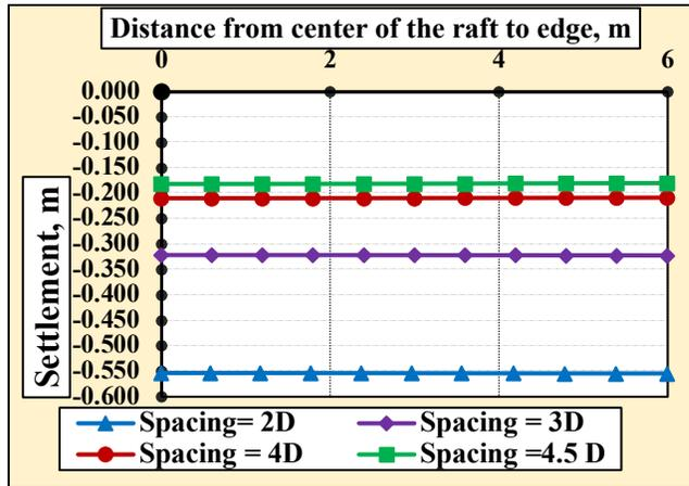
Fig. 11: Variation settlement along the centerline of a raft with the pile spacing (S).
