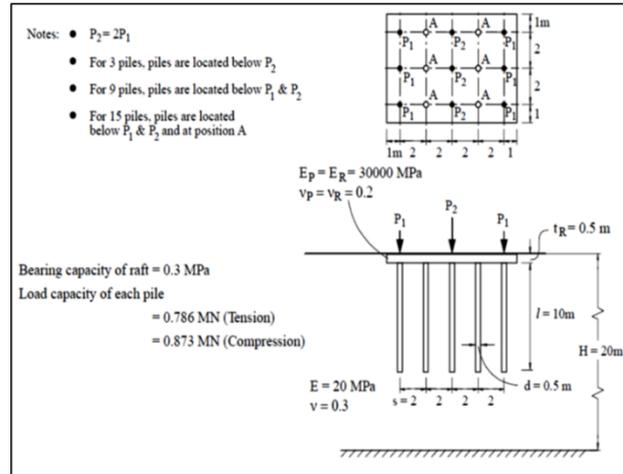
Fig. 4: Layout of piled raft example.
