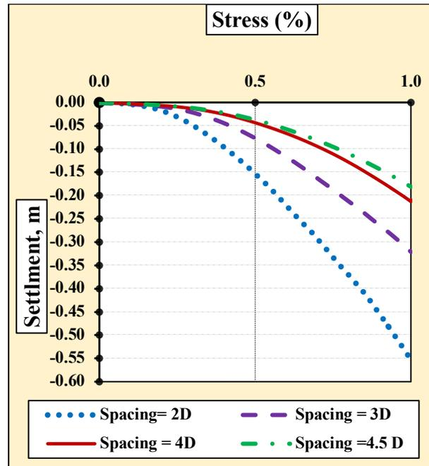
**Fig. 10:** Variation of settlement in the center of the raft with the pile spacing (S).
