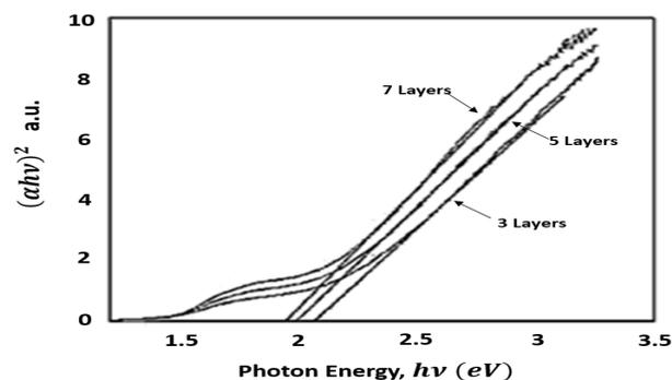
**Fig. 4:** Plots of  $(\alpha h\nu)^2$  against  $h\nu$  of  $\text{Co}_3\text{O}_4$  thin films with different layers annealed at  $350^\circ\text{C}$ .
