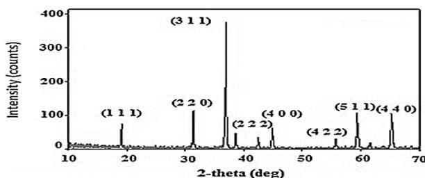
**Fig. 1:** XRD pattern of  $\text{Co}_3\text{O}_4$  thin film prepared on glass substrate and annealed at  $650^\circ\text{C}$ .
