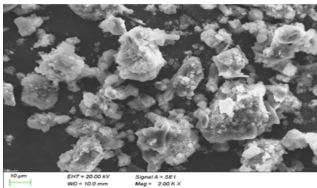
**Fig. 2:** SEM image of  $\text{Co}_3\text{O}_4$  thin film annealed at  $350^\circ\text{C}$  for 20 minutes.
