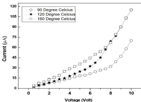
**Fig. 5:** I–V Characteristics of  $\text{Co}_3\text{O}_4$  thin film with different measurement temperatures annealed at  $350^\circ\text{C}$ .
