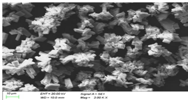
**Fig. 3:** SEM image of  $\text{Co}_3\text{O}_4$  thin film annealed at  $650^\circ\text{C}$  for 20 minutes.
