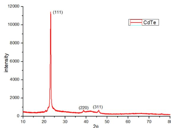
**Fig. 9:** The XRD pattern of the pristine CdTe thin film
