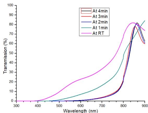
**Fig. 2:** The transmission versus wavelength curve for all the thin films of CdTe
