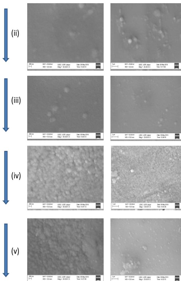
**Fig. 5:** The SEM images from RT to 4min annealing are shown in (i) to (v<sup>th</sup>) respectively
