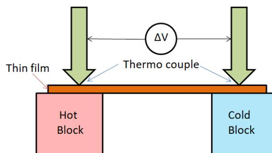
**Fig. 6:** The schematic diagram of TEP measurements
