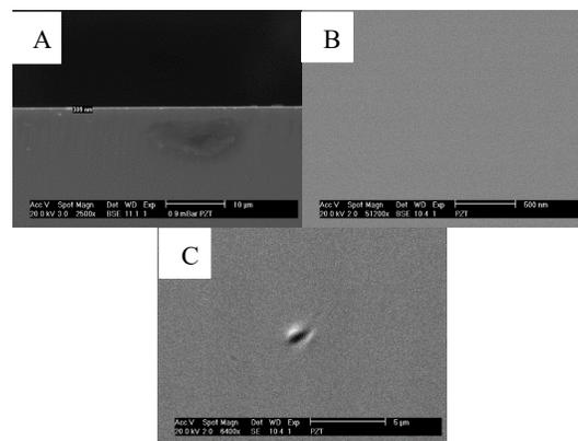
**Fig. 4:** SEM images for annealed PZT thin films A) tilted image showing 300 nm, B) high magnification image, C) low magnification image.
