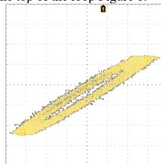
**Fig. 6:** The hysteresis loop of the annealed PZT thin film.
