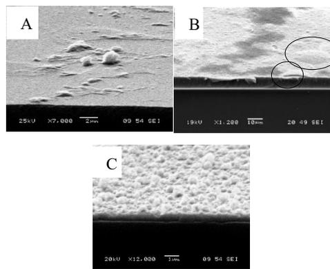
**Fig. 2:** SEM images of PZT as deposited thin films at Ar pressure of 3pa A) at 100 W, B) 150 W and C) 200W.
