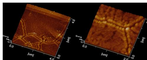
**Fig. 5:** AFM 3D images measuring the roughness of 38 to 45 nm for the annealed PZT thin films.
