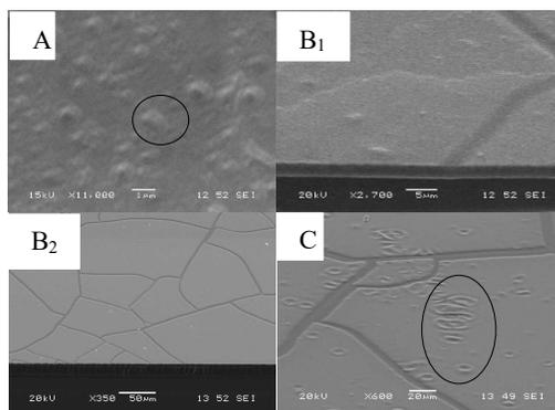
**Fig. 1:** SEM images of PZT as deposited thin films at Ar presser of 2 Pa, A) 100 W, B) 150 W and B) 200 W.
