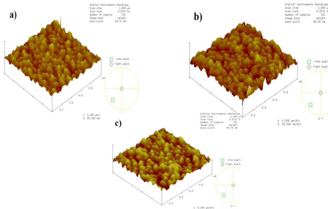
**Figure 3 :** AFM graphs of a) as-deposited b) 100 MeV oxygen irradiated CdTe thin films for the fluence  $5 \times 10^{11}$  and c) for  $5 \times 10^{12}$  ions/cm<sup>2</sup>
