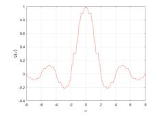
**Fig. 8:** Graph of  $g(\boldsymbol{\omega})$  in the case of  $\boldsymbol{\alpha} = 0.63$ , and  $\boldsymbol{\omega}_0 = 0$ .
