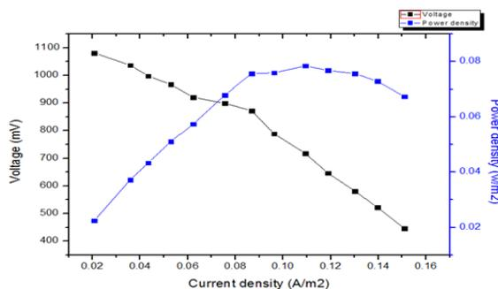
**Figure.4** Stack MFCs polarization power curve
