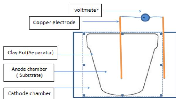
**Figure (1)** a schematic diagram of a our MFC
