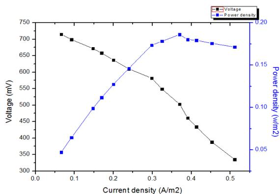
**Figure.3** large MFC polarization power curve
