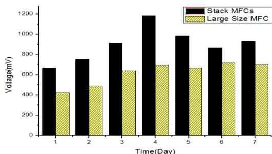
**Figure 2.** Effect of different up Scale MFC designs on production of electricity.
