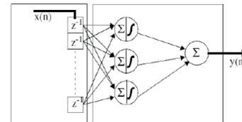
Figure 1: TDNN without feedback model
