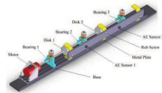
Figure 2: Rotor rub-impact testing equipment
