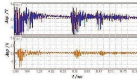
Figure 3: The measured acoustic emitted signals received by sensor
