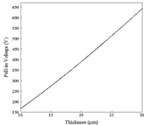
Fig. 5: Pull-in voltage versus micro-beam thickness
