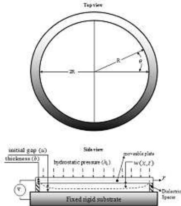
Fig. 1: Schematic illustration of micro circular plate actuator system.
