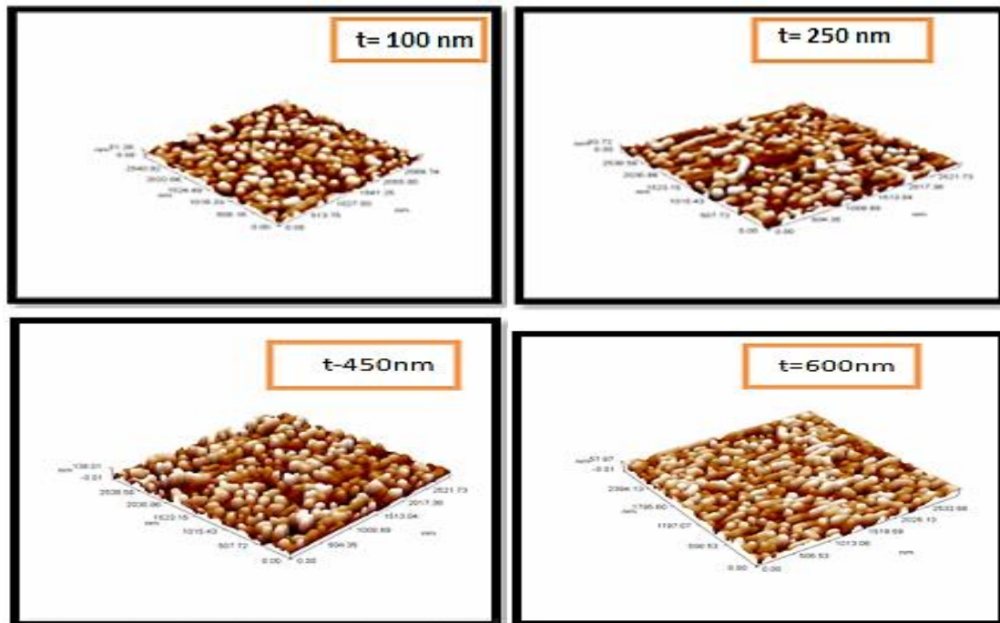
Figure 2. AFM images for SnS films at different thickness
