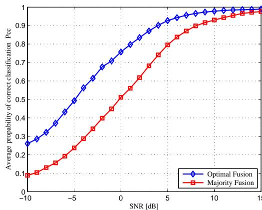
**Fig. 5:** Average probability of correct classification versus SNR at different fusion scenarios.
