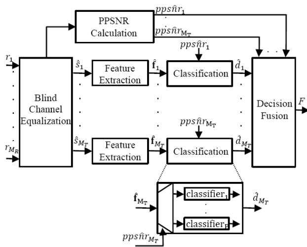
**Fig. 1:** A block diagram of the proposed AMC algorithm.
