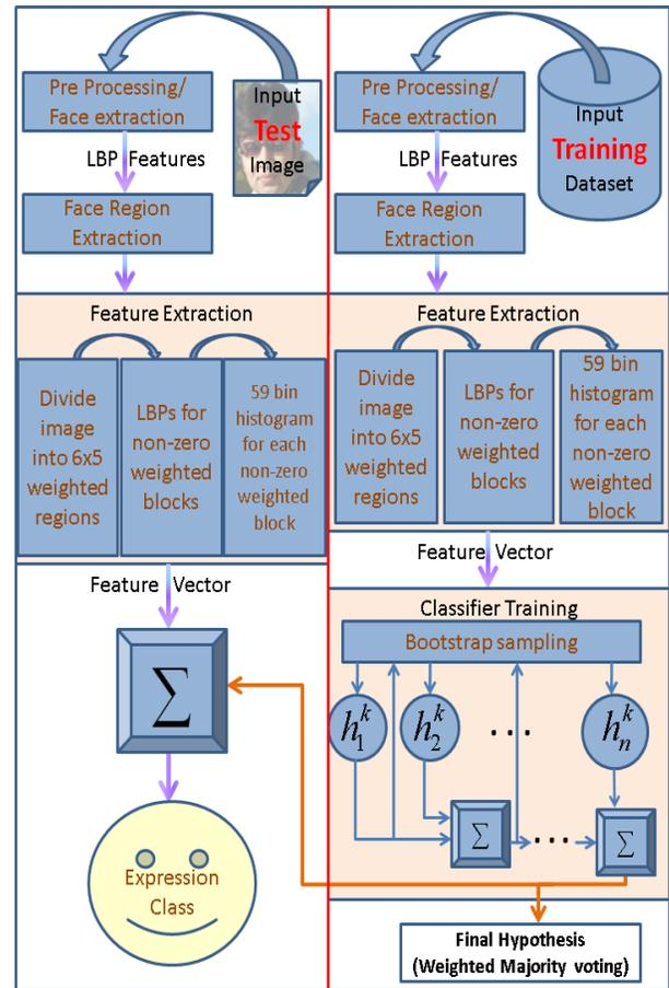
**Fig. 2:** Block diagram of the proposed system: right side represents the training process and left side represent the testing process
