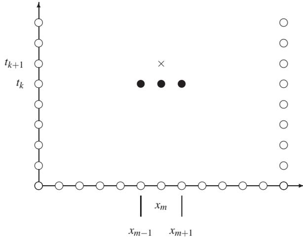
**Fig. 1:** Forward-difference stencil of the finite-difference method (7) at the time  $t_k$  around the node  $x_m$ . The black circles represent the known approximations to the exact solution at time  $t_k$ , and the cross denotes the unknown approximation at time  $t_{k+1}$ .
