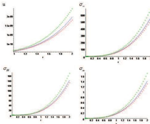
**Fig. 3:** Effect of  $H_\phi$  on displacement and stresses displacement with radius  $r$ ,  $H_\phi = 0.3$ "Green",  $H_\phi = 0.5$ "Blue",  $H_\phi = 0.7$ "Red".
