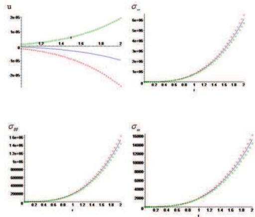
**Fig. 4:** Effect of  $\tau_0$  on displacement and stresses displacement with radius  $r$ ,  $\tau_0 = 0.1$ "Green",  $\tau_0 = 0.3$ "Blue",  $\tau_0 = 0.5$ "Red".
