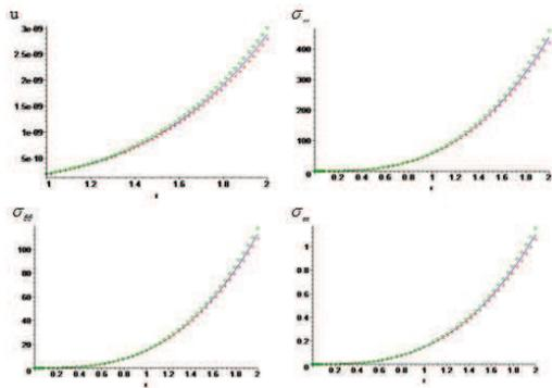
Fig. 6: Effect of  $\Omega$  on displacement and stresses displacement with radius  $r$ ,  $\Omega = 0.3$  "Green",  $\Omega = 0.5$  "Blue",  $\Omega = 0.7$  "Red".
