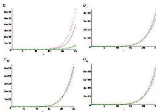
Fig. 9: Effect of  $\Omega$  on displacement and stresses displacement with radius  $r$ ,  $\Omega = 0.3$  "Green",  $\Omega = 0.5$  "Blue",  $\Omega = 0.7$  "Red".
