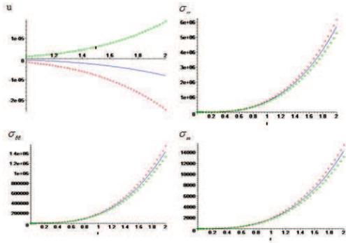
**Fig. 1:** Effect of  $\tau_0$  on displacement and stresses displacement with radius  $r$ ,  $\tau_0 = 0.1$ "Green",  $\tau_0 = 0.3$ "Blue",  $\tau_0 = 0.5$ "Red".
