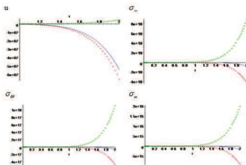
Fig. 8: Effect of  $\tau_0$  on displacement and stresses displacement with radius  $r$ ,  $\tau_0 = 0.1$  "Green",  $\tau_0 = 0.3$  "Blue",  $\tau_0 = 0.5$  "Red".
