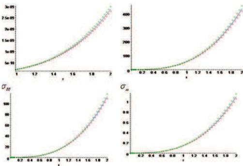
**Fig. 2:** Effect of  $\Omega$  on displacement and stresses displacement with radius  $r$ ,  $\Omega = 0.3$ "Green",  $\Omega = 0.5$ "Blue",  $\Omega = 0.7$ "Red".
