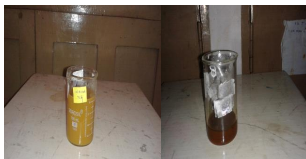
Figure 3: Formation of copper nanoparticle a) presence of PEG 6000 and b) absence of PEG 6000 for the composition (1:3) (extract: \text{CuSO}_4 )
