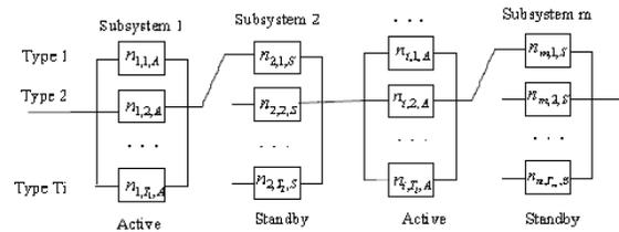
**Fig. 1:** General series-parallel system with a choice of redundancy strategy
