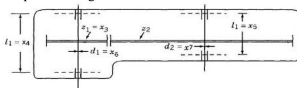
Figure 2: Speed reducer design [9]
