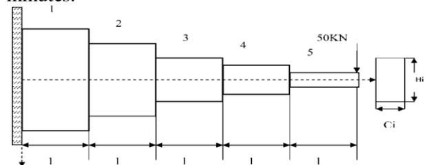
Figure 1: A stepped cantilever beam [35]
