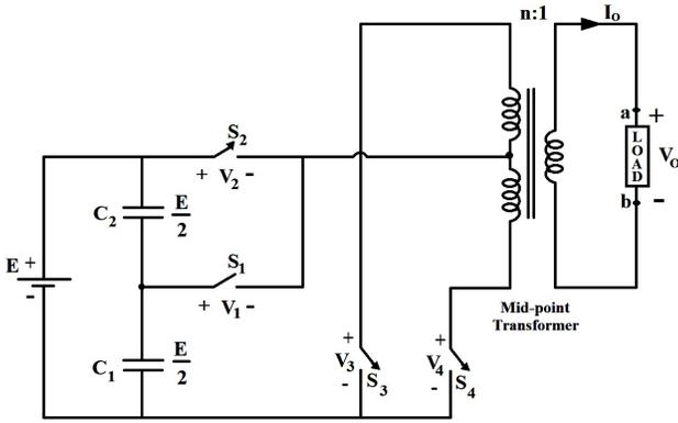
**Fig. 1:** Circuit diagram of the proposed push-pull multilevel inverter topology.
