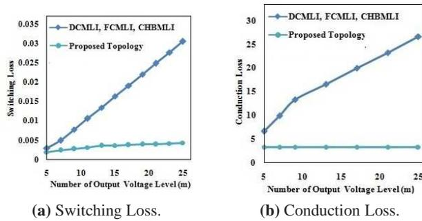
**Fig. 5:** Comparison of the losses of the proposed topology and other classical topologies.
