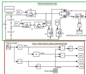
**Fig. 6:** Simulink model of the proposed push-pull five level inverter with the novel PWM control signal generation unit.
