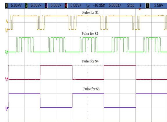
**Fig. 8:** Experimental Pulse pattern.
