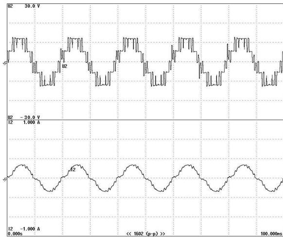
Fig. 12: Experimental Output Voltage and Output Current (R-L load).
