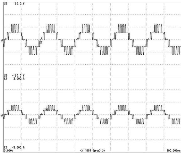
Fig. 10: Experimental Output Voltage and Output Current waveform (R load)
