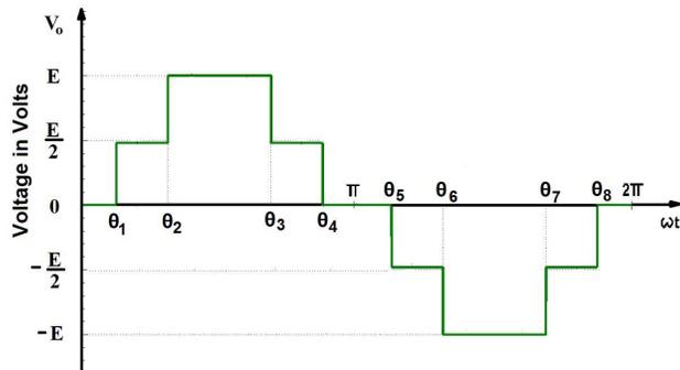
**Fig. 2:** Five level inverter stepped output voltage.
