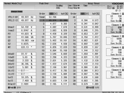
Fig. 15: Power quality analyser harmonic content for R-L load.
