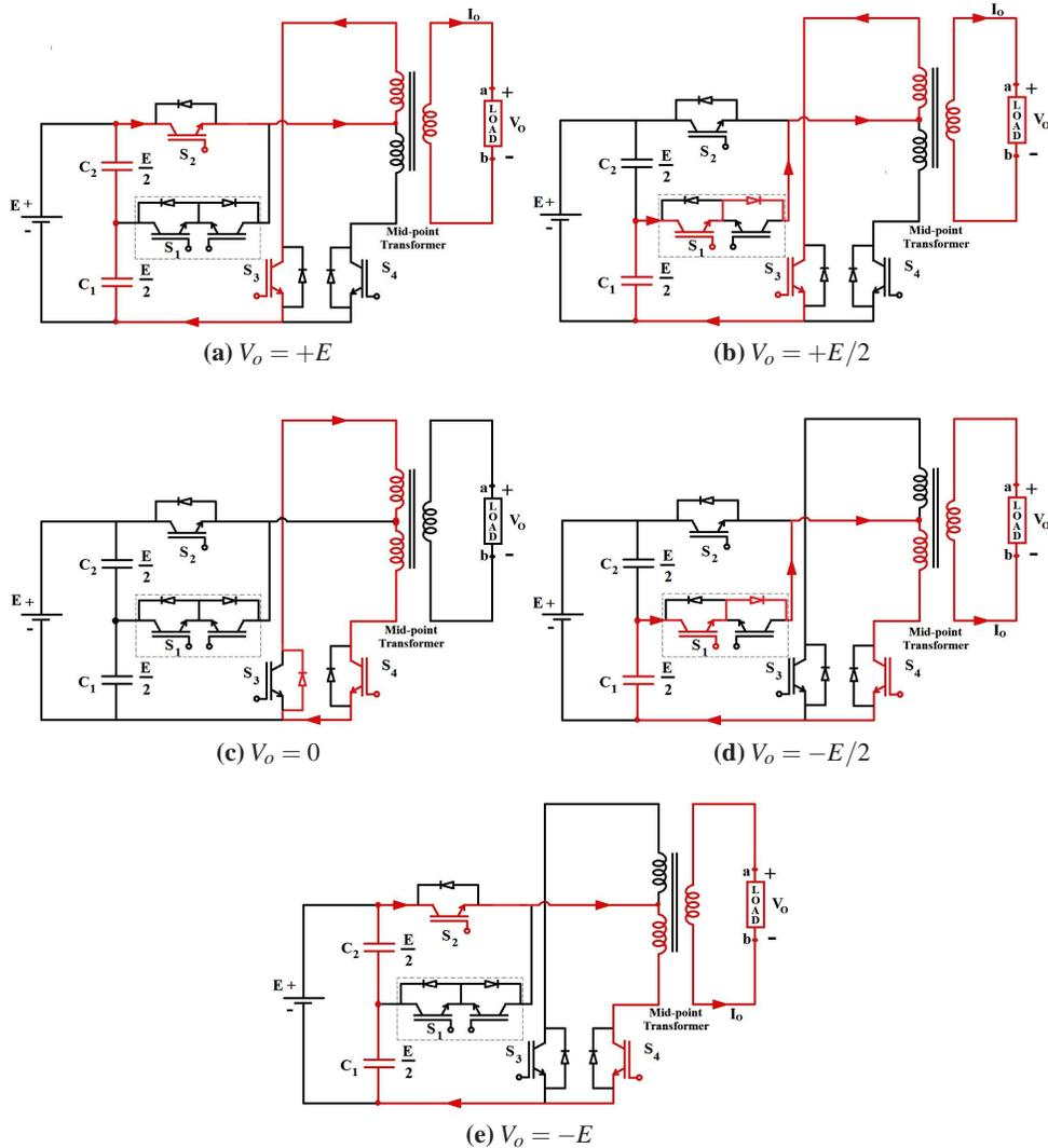
**Fig. 3:** Modes of operation with current path.
