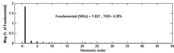
Fig. 13: MATLAB Output Current harmonic spectrum of the proposed push-pull five Inverter with R-L Load (without filter).
