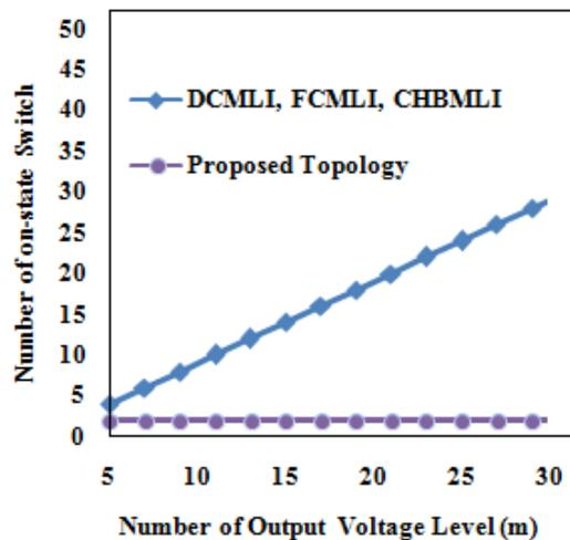
(d) On-state switches with respect to number of levels.
