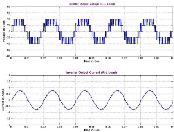
Fig. 11: Simulated Output Voltage and Output Current (R-L load).
