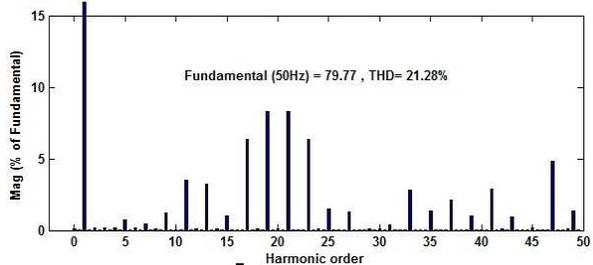
Fig. 14: Simulated voltage harmonic spectrum of the proposed push-pull five Inverter with R-L Load (without filter).
