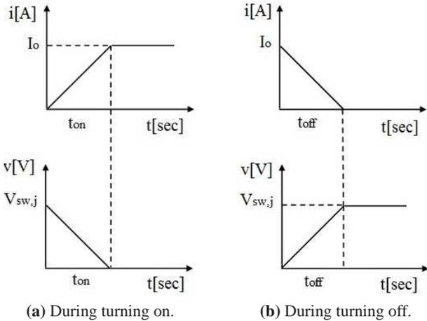
**Fig. 4:** Current and voltage waveforms of a switch.
