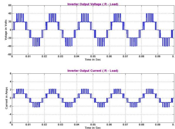
**Fig. 9:** Simulated Output Voltage and Output Current Waveform (R load).
