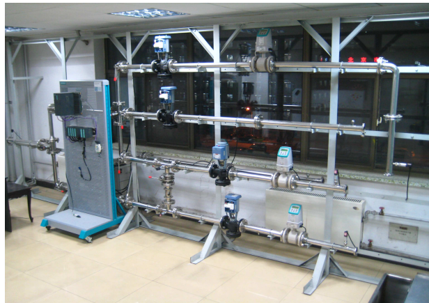
Fig. 8: Photo of the Complex Pipe Network Pressure and Flowrate Monitoring Experiment Device
