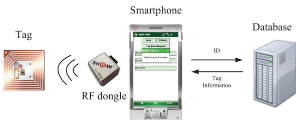
**Figure 3** : Experimental testbed is set up as follows: one desktop computer is configured as a database server. Nesslab’s 900 MHz -UHF RF reader dongle as a RFID reader and Power IDs EPC Gen-2 tags are used.
