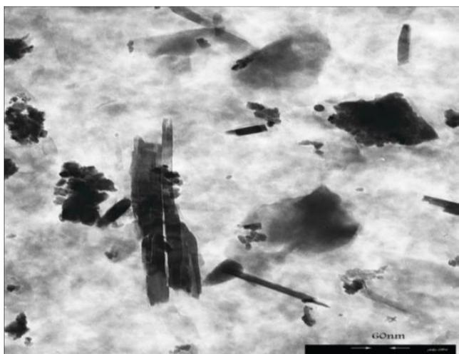
**Figure 1.** Transition Electron Microscopy Image of Bentonite
