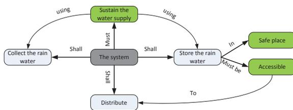
**Fig. 8:** Modelling the requirements and attributes of water system design using olog.
