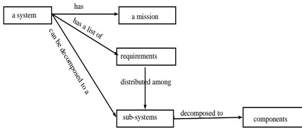
**Fig. 6:** An object can have many aspects, as for example, a system has a mission, a set of requirements and can be decomposed to sub-systems.
