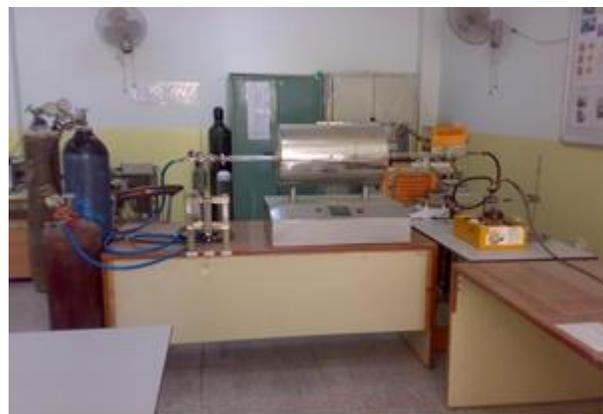
Fig.1: photograph of setup CVD.
