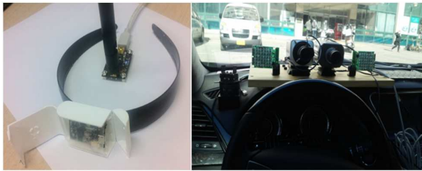
Fig. 8: Wireless Gyro-sensor module mounted in a white box and its receiver (Left) and cameras and other setup installed in the vehicle (Right)
