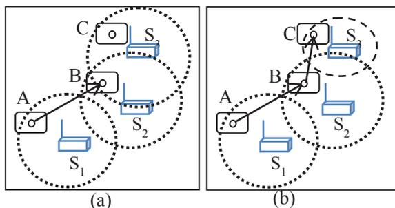
**Figure 1** The illustration of the power level setting affecting the data mule path planning.
