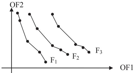
**Figure 2** Illustration of a front set  $F$ , where  $F = F_1, F_2, F_3$ . Each point represents one feasible solution in one front in the 2-dimensional space.  $F_1$  is the most efficient front, which is the result of the Data Mule Path Planning Algorithm. The ranks of the three fronts ordered from highest to lowest are  $F_1, F_2$ , and then  $F_3$ .
