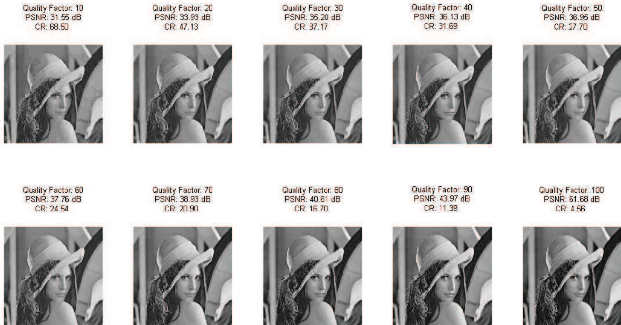
Fig. 4: Illustration of results of the proposed scheme for various QF and their PSNR in dB and CR values
