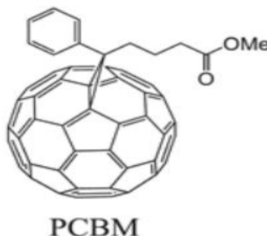
Fig. 1: The organic structure of PCBM.[13]
