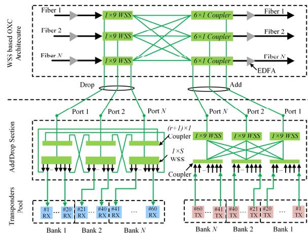
**Fig. 1:** CDC ROADMs with OXC and add/drop sections where the nodal degree  $N$  equals 3, the connecting branches  $r$  is  $N-1$ , here equals 2,  $S$  equals 23, 40 wavelengths per fiber and 50% add/drop ratio, RX: Receiver (in blue), TX: Transmitter (in red).
