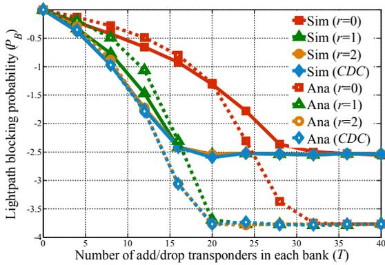
**Fig. 3:** The light-path blocking performance of the Italy network. (Ana: Analysis (dashed curve), Sim: Simulation (solid curve), 1.5 Erlang per node pair,  $r$  denotes the number of connecting branches, CDC case: where  $r$  equals  $N-1$ , where the max ( $N_i$ ) is 9).
