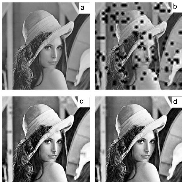
**Figure 4** Inpainting results comparison of TV wavelet and Model III on lena. (a) Original image; (b) Received image with 10% wavelet coefficients loss (PSNR=17.1900); (c) TV inpainting (PSNR=24.2052); (d) Model III (PSNR=25.1206,  $\alpha = 1.4$ )
