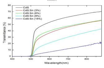
Fig.3b.The optical transmission spectra of the CdS:Sn thin films.
