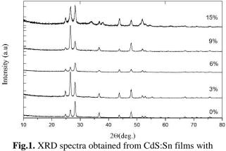
**Fig.1.** XRD spectra obtained from CdS:Sn films with varying vol % of Sn.
