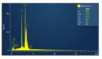
Fig.2. EDX micrograph of CdS:Sn by the 15% Sn volume percentage thin film on glass substrate.
