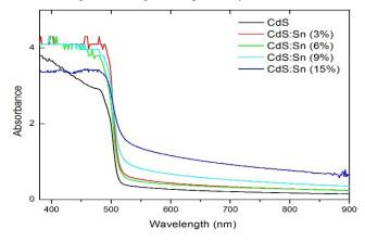
Fig.3a.The optical absorbance spectra of the CdS:Sn thin films.
