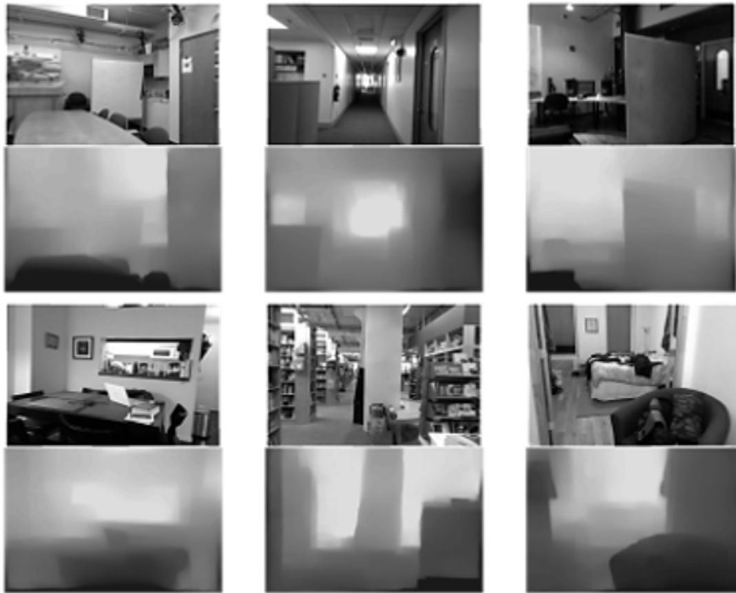
Fig. 2: Depth output result using our proposed model from the NYU V2 dataset
