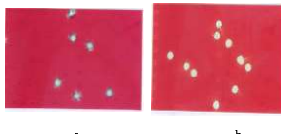
Fig. 3: Photomicrograph of 2 MeV \alpha -tracks in LR-115 detectors, etched in 2.5N NaOH at 50^\circ\text{C} for (a) h = 5\ \mu\text{m} and (b) 6\ \mu\text{m} , without pre-sparking.
